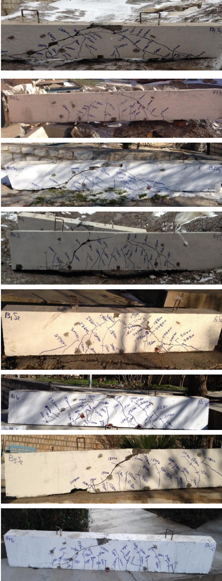
Fig.5 Crack Patterns of Tested Beams
