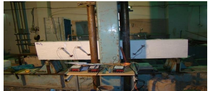
Fig.2 LVDT Instruments and Their Location
