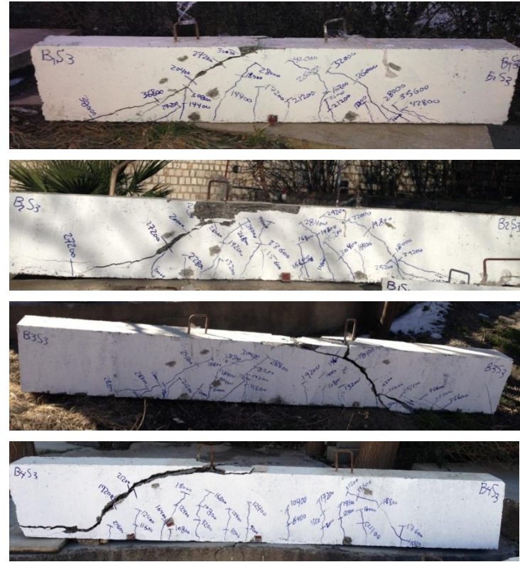
Fig.5 Crack Patterns of Tested Beams
